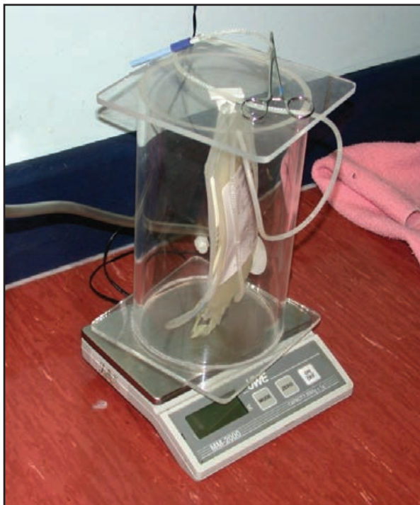
34.7 Vacuum-assisted blood collection chamber, and scale used to determine collection volume by weight.
