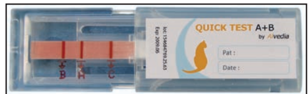
33.5 The Alvedia Quick Test system for feline blood typing. The left-hand end of this immunochromatographic strip has been inserted previously into a suspension of feline blood cells, and these have migrated through the strip matrix to interact at specific points with typing reagents (positions B and A). A control (C) reaction is also included. This test is validated by the presence of the control line and shows that the cat is of blood type AB.
